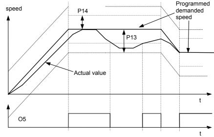
Positioning and control functions Speed monitoring in speed control mode (P93="4")
